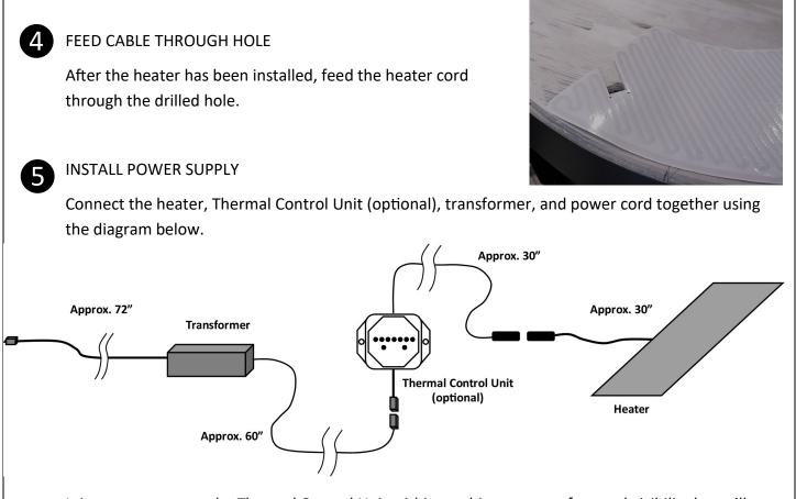
It is common to put the Thermal Control Unit within a cabinet or out of normal visibility but still accessible for periodic use. The Thermal Control Unit can be mounted onto the inside wall of a cabinet with the screws provided. The transformer typically lies in a cupboard or in the bottom of the cabinet. The transformer may feel warm to the touch (or a bit hot in some cases)—this is normal.
