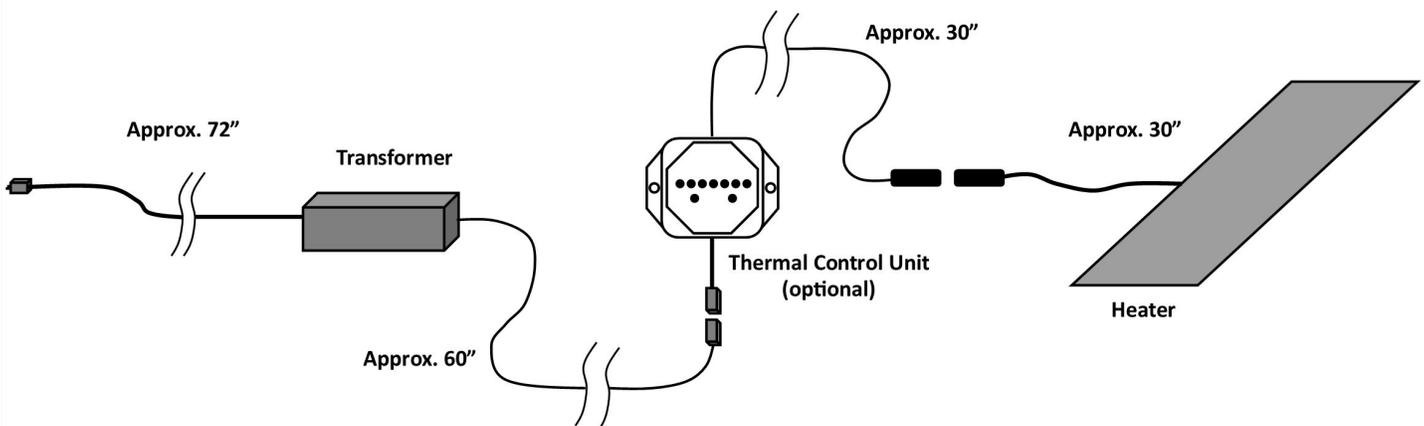
It is common to put the Thermal Control Unit within a cabinet or out of normal visibility but still accessible for periodic use. The Thermal Control Unit can be mounted onto the inside wall of a cabinet with the screws provided. The transformer typically lies in a cupboard or in the bottom of the cabinet. The transformer may feel warm to the touch (or a bit hot in some cases)—this is normal.
