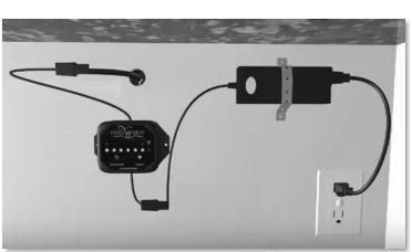
onto the cabinet wall. Secure the wires using the mating Velcro piece. If the Velcro patches do not stick to your cabinet wall, use the strap included. Cut the strap to the desired length and drill the screws into the cabinet wall to secure your transformer.
