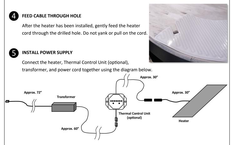
**IMPORTANT**: If the FeelsWarm system that has been purchased involves multiple transformers and/or multiple heaters, each transformer plug and each heater cable will have a numerical tag with matching code numbers. It is extremely important that the correct transformer is plugged into its correlating heater.
