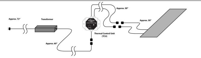
It is common to put the Thermal Control Unit within a cabinet or out of normal visibility but still accessible for periodic use. The Thermal Control Unit can be mounted onto the inside wall of a cabinet with the screws and strap provided. The transformer typically lies in a cupboard or in the bottom of the cabinet. The transformer may feel warm to the touch (or a bit hot in some cases)—this is normal.
