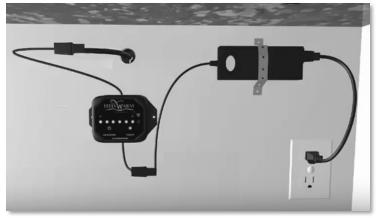
onto the cabinet wall. Secure the wires using the mating Velcro piece. If the Velcro patches do not stick to your cabinet wall, use the strap included. Cut the strap to the desired length and drill the screws into the cabinet wall to secure your transformer.
