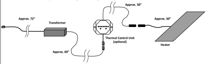
**IMPORTANT**: If the FeelsWarm system that has been purchased involves multiple transformers and/or multiple heaters, each transformer plug and each heater cable will have a numerical tag with matching code numbers. It is extremely important that the correct transformer is plugged into its correlating heater.
